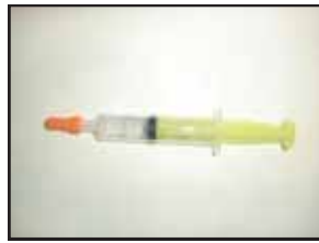
Figure 3: (Above) Using cap for preventing leaking.
